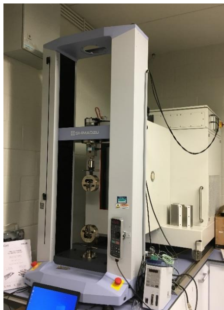
Figure 5. Single lap shear testing setup
