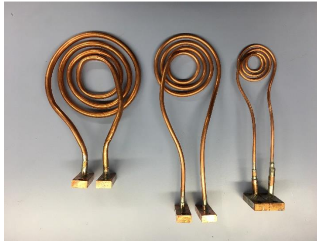
Figure 4. Flat spiral (pancake) coils used
