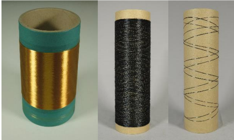
Lignin precursor fibers spun from water, stabilized and carbonized continuous fibers
