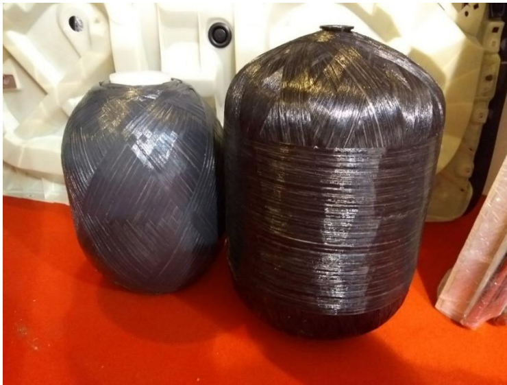
Figure: Thermoplastic composite pressure vessels. Thermoplastic composite tape wound on PP (left) and steel (right) liners
